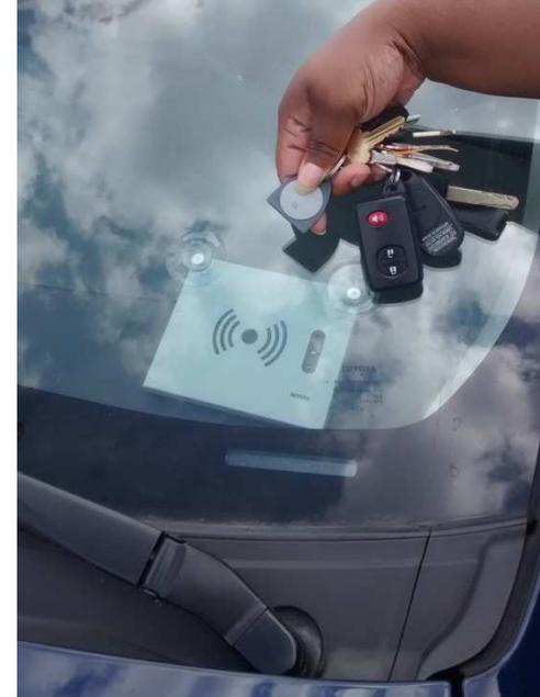
If the car still won't lock using your HOURCAR fob, please make sure that you've returned the car keys to the keypad in the glove box. If the keypad fob is not reinserted into the keypad, the reader will not lock the car doors when you swipe your HOURCAR fob. You may be charged \$100 if you take the car keys with you! Avoid the fee – leave the key!
