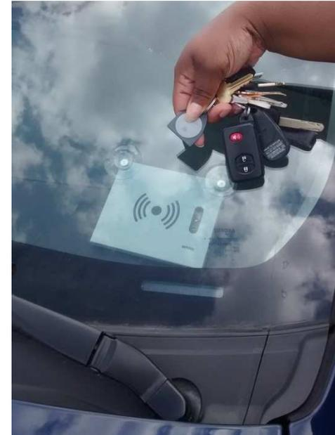
You will find the fob reader in the window near the driver's side of the vehicle – that hasn't changed. Hold your fob against the window briefly to trigger the reader. The yellow light on the reader will illuminate— this means that your fob has been read and you may remove it. If the red light flashes, it has not read the fob yet. When the green light illuminates, you'll hear the doors unlock. Go ahead and hop into the car!
