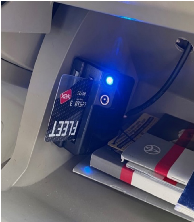
Blue LED light indicating the key is removed (the keyfob is not in the fob holder.)
