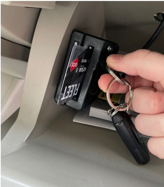
Remove the key from the holder by gently pulling the fob out of the jack
